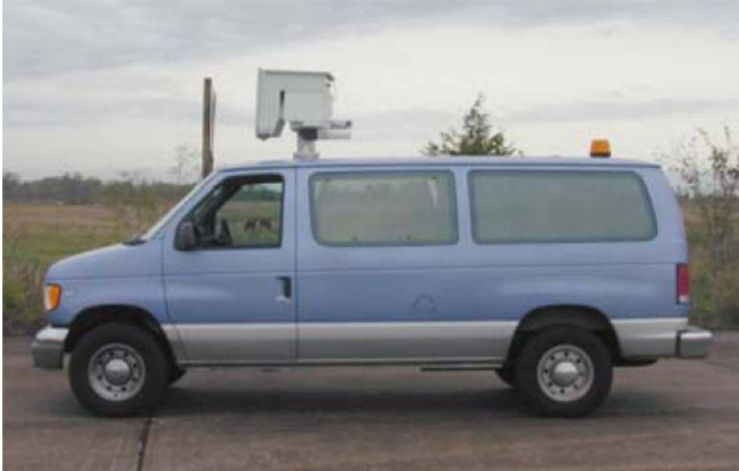
Figure 2. One of the Four FHWA Mobile Sign Retroreflectivity Vans (circa 2002)
